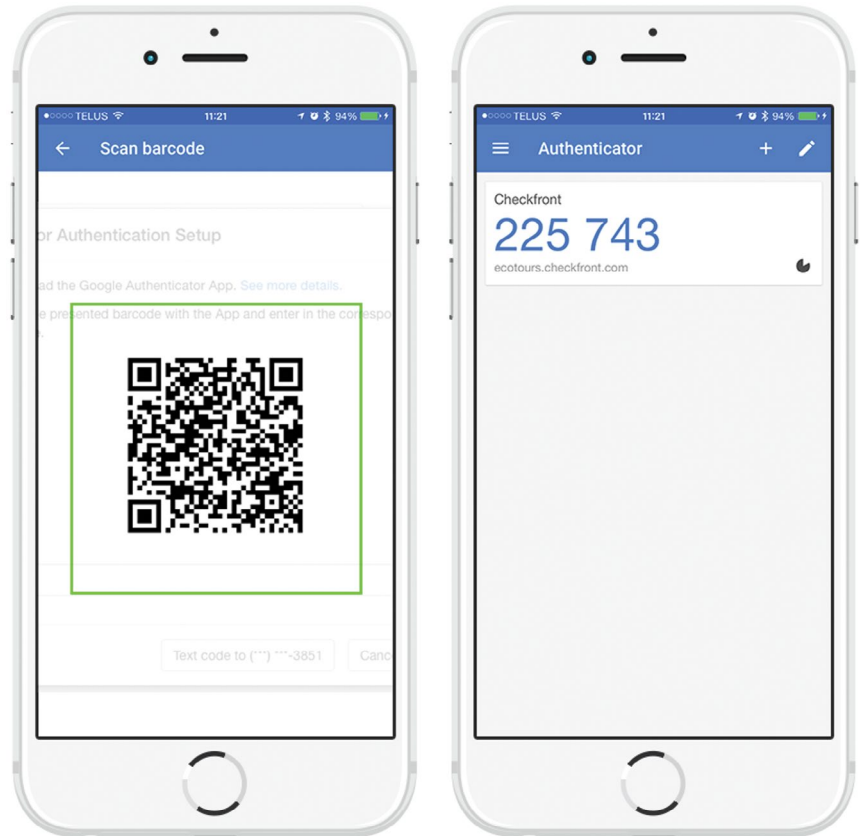
Figure 5 Implementation of 2-factor authentication by using a mobile application instead of SMS Source: https://medium.com/
